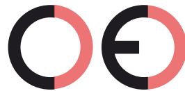
False CE Mark (too far)
